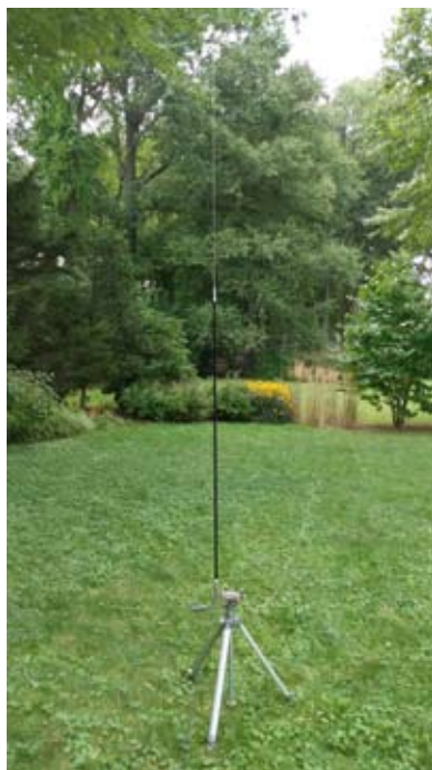
Hamstick on Tripod and Clamp Mounts with push-on counterpoise wire connections
