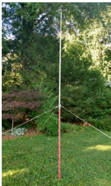
Pole Pruner 20m Antenna with 3 guy lines to tent stakes
