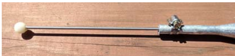
Tunable Tip can be adjusted in/out for the lowest SWR
