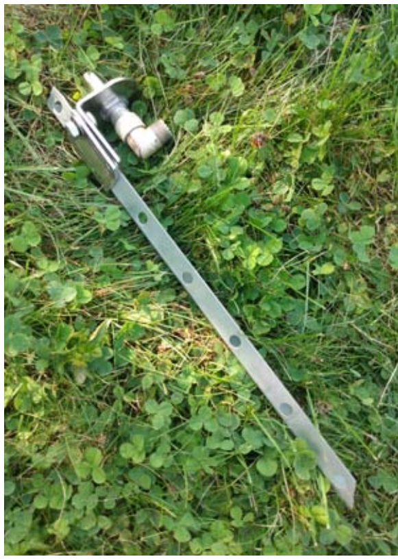
Spike Mount with SO-239 connection and right angle adapter
