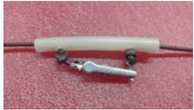
Single Alligator Clip Link wires secured to plastic tubing with knots
