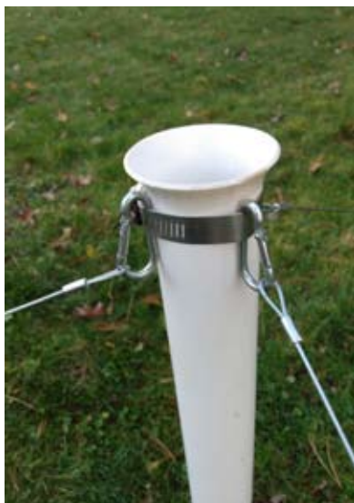
Snap Links at Top of Spike secured with hose clamp
