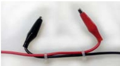
Dual Alligator Clip Link wires secured with zip ties as shown or a square knot
