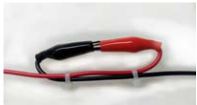
Dual Alligator Clip Link wires secured with zip ties as shown or a square knot
