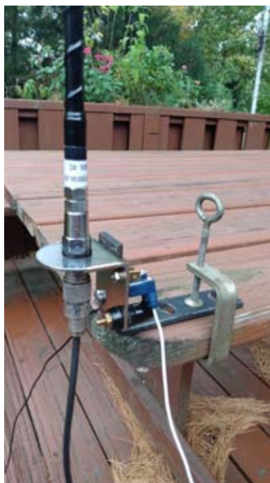
Hamstick on Tripod and Clamp Mounts with push-on counterpoise wire connections
