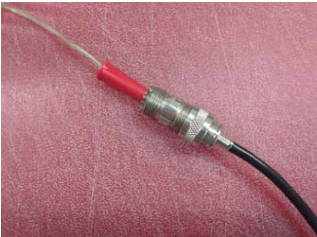
Linked Vertical Feedpoint with double-female connector
