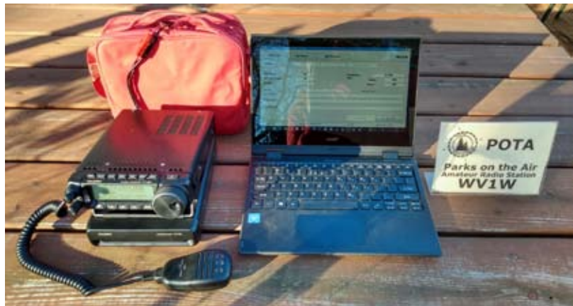
Yaesu FT-891 with FC-50 tuner fits conveniently under radio
