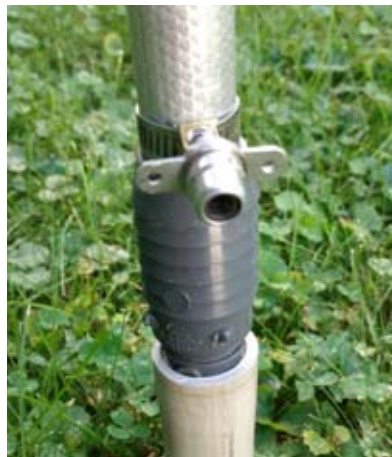
RCA Feedpoint with Tabs for Counterpoise Wires
