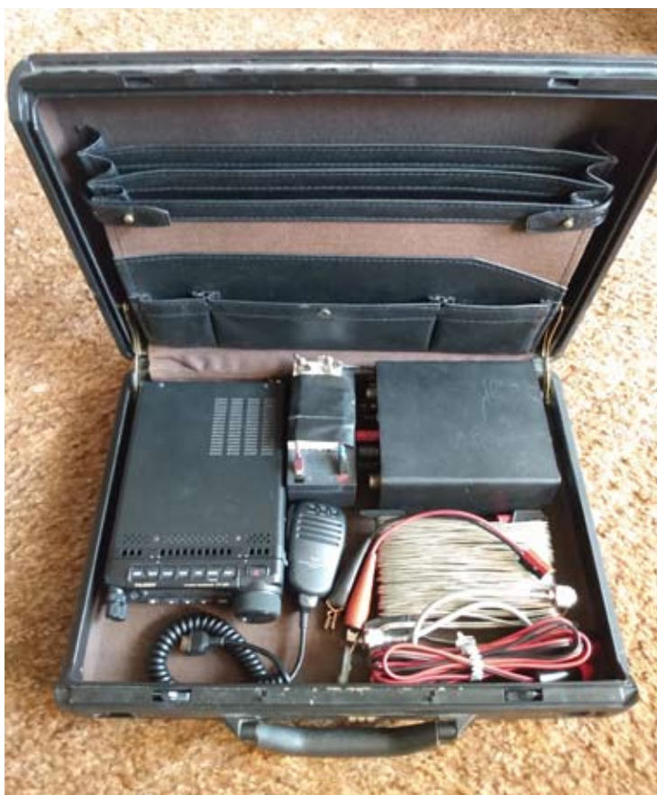
Complete Station Packed in a Briefcase rig, tuner, battery, mic, and antenna
