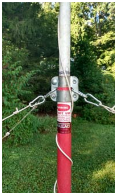
Pole Pruner 20m Antenna with 3 guy lines to tent stakes
