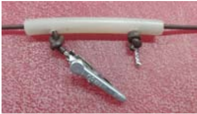
Single Alligator Clip Link wires secured to plastic tubing with knots
