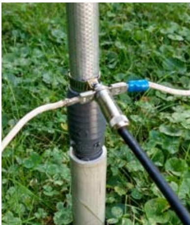
RCA Feedpoint with Tabs for Counterpoise Wires
