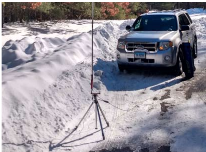
Tent Pole Vertical on Tripod Mount
