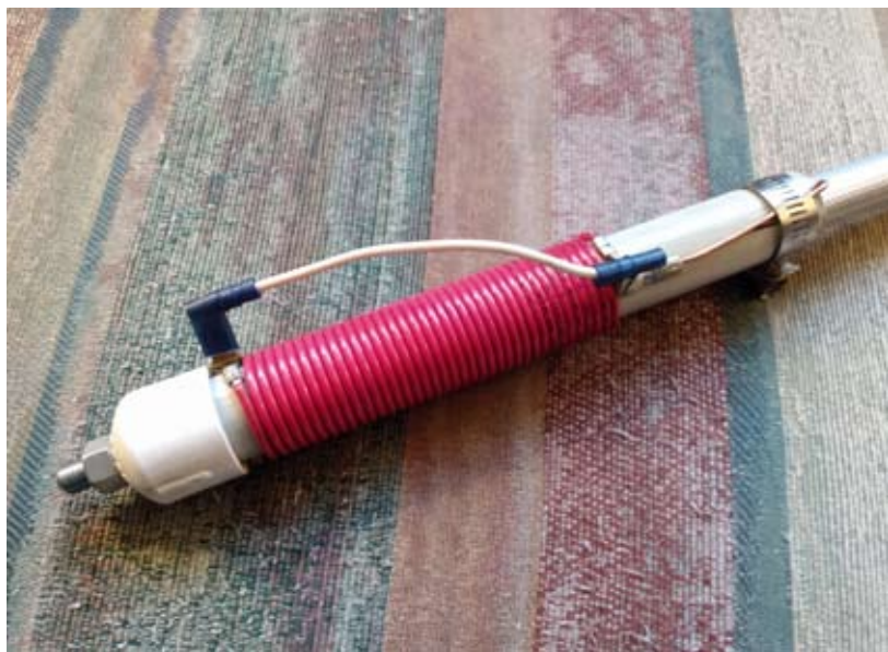
40m Loading Coil with easily removable jumper for 20m
