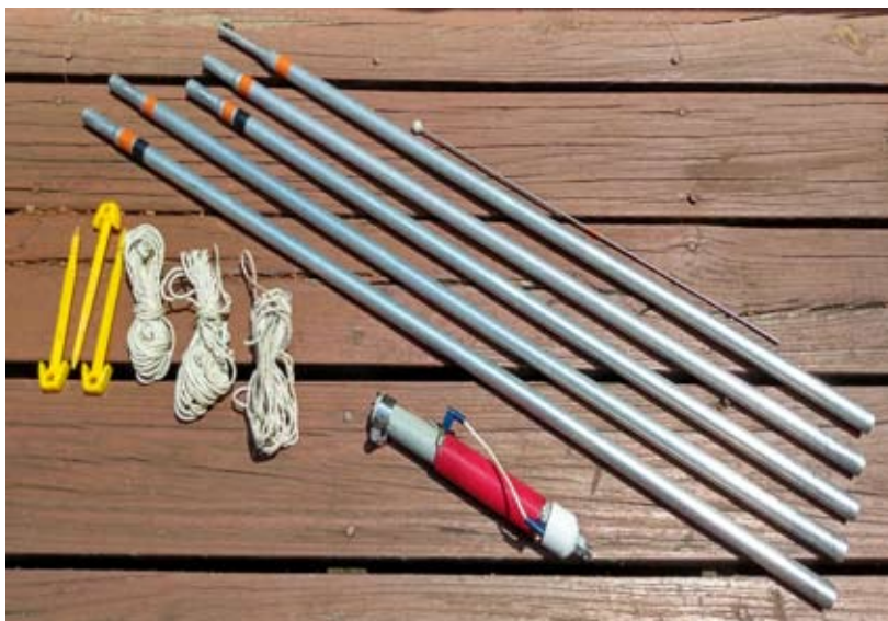
Tent Pole Antenna Parts with 40m coil and guy system for windy days
