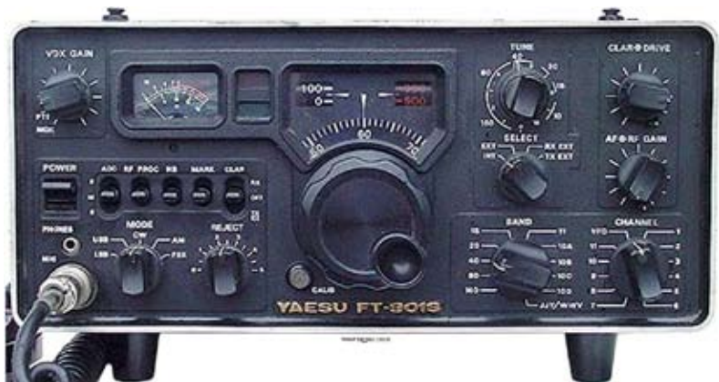
Yaesu FT-301S 10-watt QRP HF Transceiver
