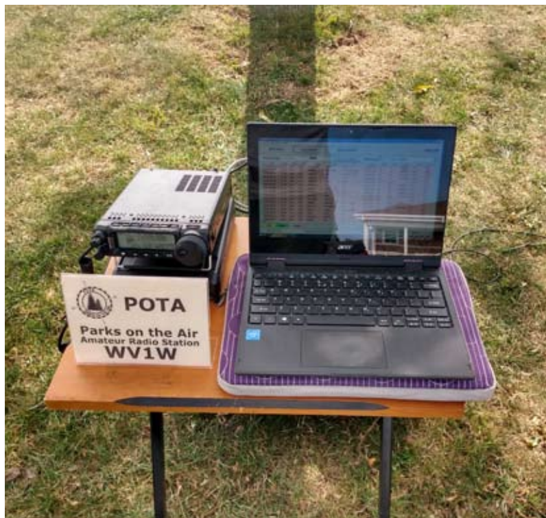
Portable Station: FT-891 & Small Laptop Computer 12-volt battery is out of sight on the ground
