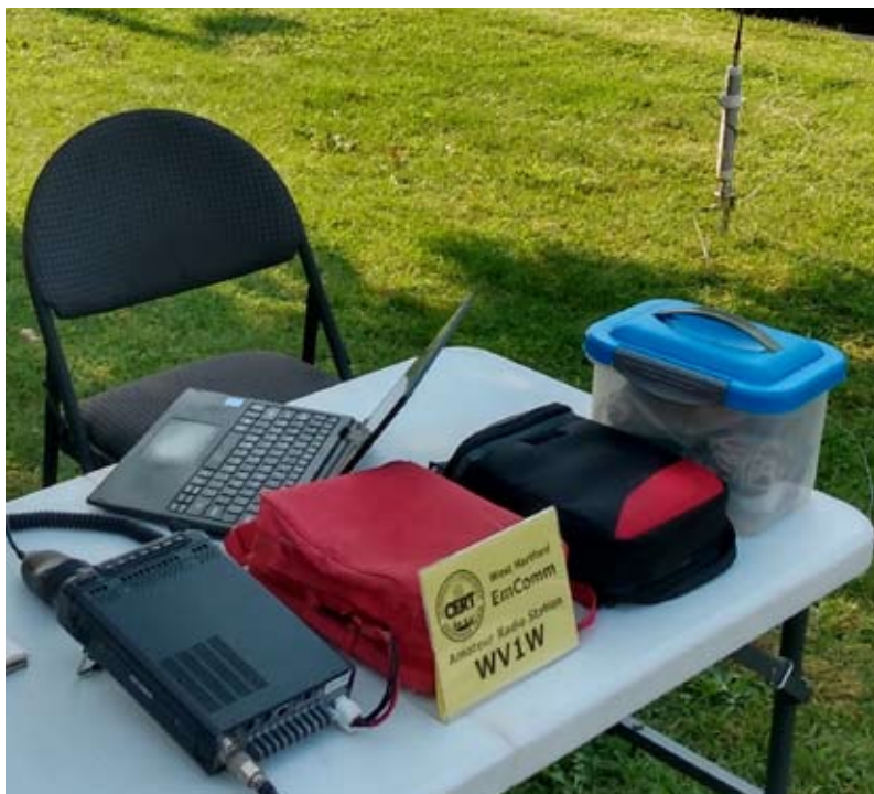
FT-891 with Stake-Mounted WRC Antenna
