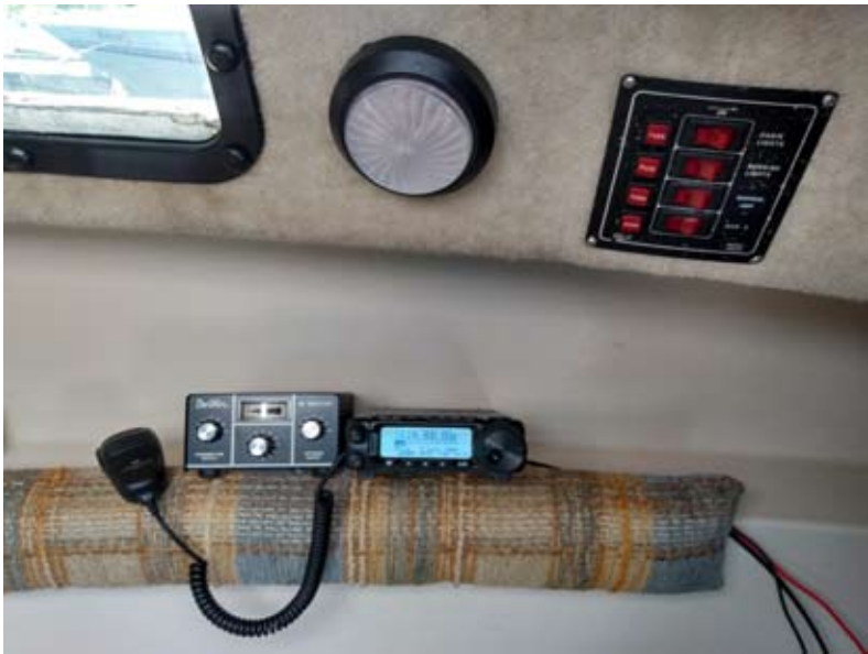
HF Station in the Cabin Dentron tuner with Yaesu FT-891 transceiver
