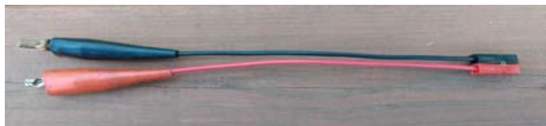
Battery Clips to Powerpoles® Adapter for running a rig directly from the car's battery
