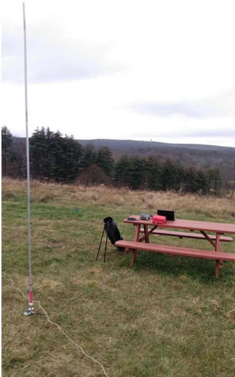
Tent Pole Vertical Antenna Deployed Auerfarm State Park Scenic Reserve (US-9896)
