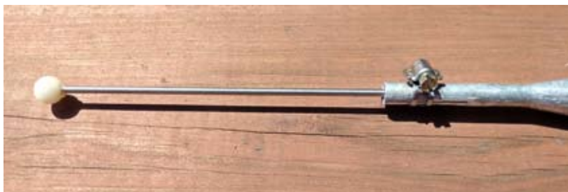
Tunable Tip can be adjusted in/out for the lowest SWR
