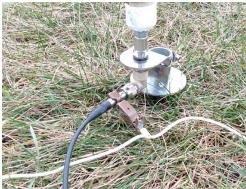
Radials Clipped to Coax Connector normally 4 are used but just 2 can work just fine
